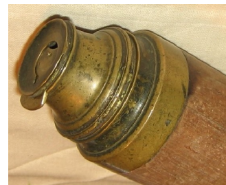
Left: Eye piece , with the sliding brass cover in the open position.
