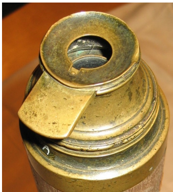
Left: Eye piece , with the sliding brass cover in the open position.
